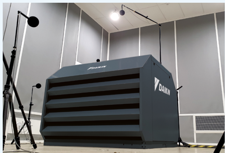
Sound power level measurement in acoustic chamber
